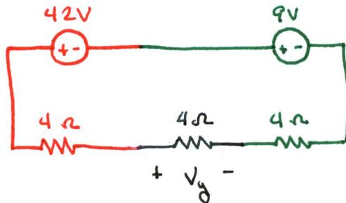
$$V_y = \frac{4\Omega}{4\Omega + 4\Omega + 4\Omega} (42V + 9V) = 17V$$
